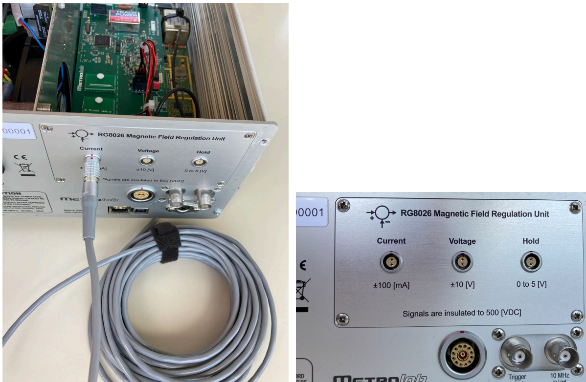
RG8026 Magnetic Field Regulation Unit (board, back panel and cable).
