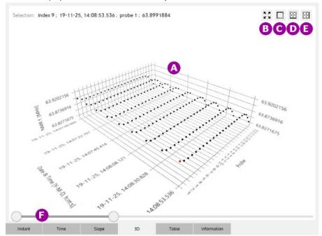
A. Display measurement **results** as a 3D plot. Depending on the operating mode, the X axis can be time or position. The Y axis is probe number. The Z axis is the NMR measurement result in MHz or Tesla. See the information on a specific operating mode using this kind of plot for more details on X-Y-Z.
