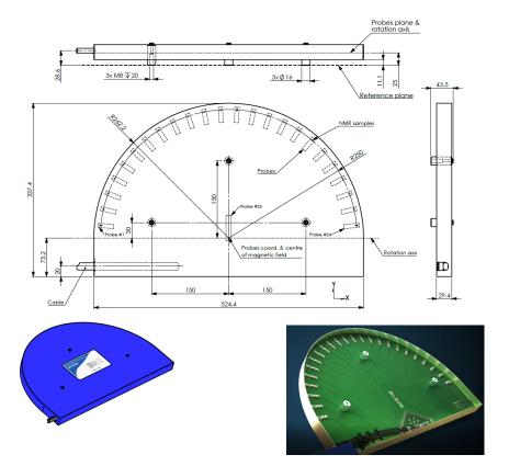
Custom Probe-Array -MFC9046, model HM24-1-250 212.4 x 29.4 x 273.4 mm
