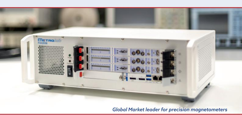
The Fast Digital Integrator FDI2056 is the world's fastest and most sensitive voltage integrator. Plug in a sense coil, and for the first time it is possible - even easy - to measure fast, low-level magnetic field disturbances such as eddy currents in a switched magnet.
