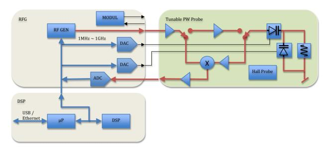
Figure 5. PT2026 functional block diagram.
