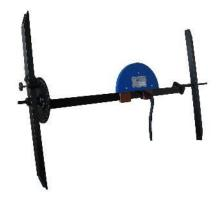
Figure 4. The Magnetic Field Camera probe array:
