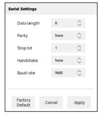
If a MFC3045 instrument is connected in MFCTool, new serial settings are directly applied to instrument when pressing "Apply". Wait few seconds for the MFC3045 to be reconfigured and restarted.
