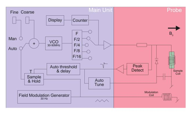
Figure 3. PT2025 functional block diagram.
