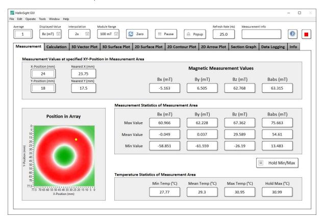
Measurement Values at specified XY-Position in Measurement Area
