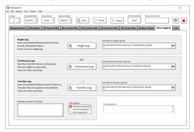
Single Log: The single log saves all measurement and calculated data to a file as it is shown in the visualization and analysis tabs. Data are saved with set *Interpolation* and Zero function. The measurement is saved once when the Single Log button is pressed.
