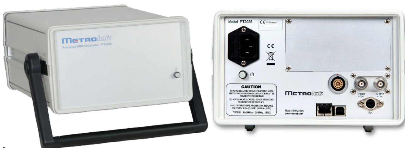
PT2026 desktop main unit, front and back panel
