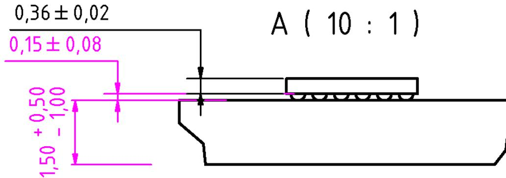
Every FH5401c sensor contains two 3-D Hall sensors (pixels) for vectorial measurement of magnetic fields. Geometrical dimensions of the sensor and the position of the actual sensitive sensor area can be extracted from following figure and table.
