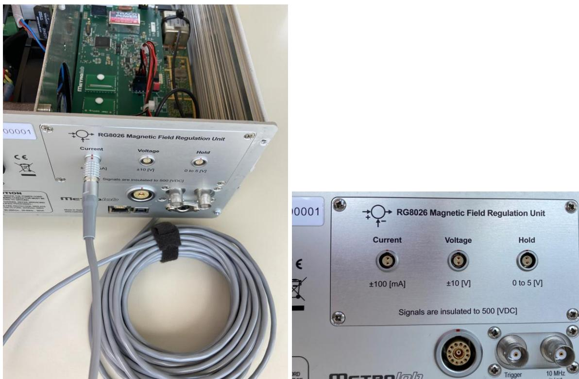
RG8026 Magnetic Field Regulation Unit (board, back panel and cable).
