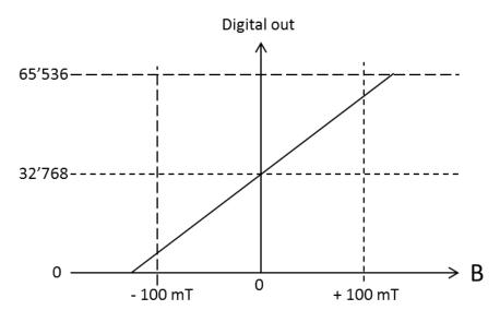
Figure 16. Output of one particular axis as a function of field strength.
