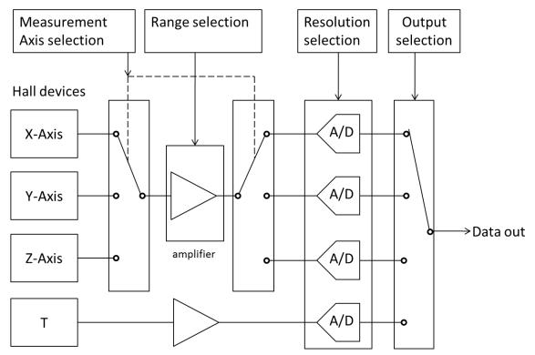
Figure 8. Block diagram of the signal conditioning – digital mode
