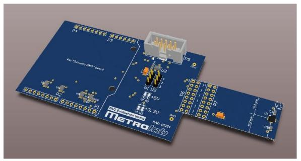
Figure 18. MagVector MV2 Evaluation Kit test board.
