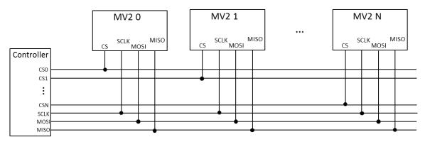
Figure 10. Parallel connection of MagVector MV2s
