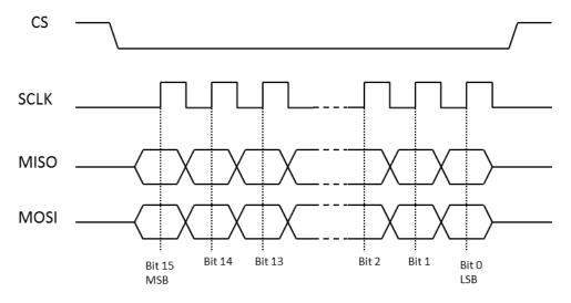
Figure 11. Timing diagram of one word
