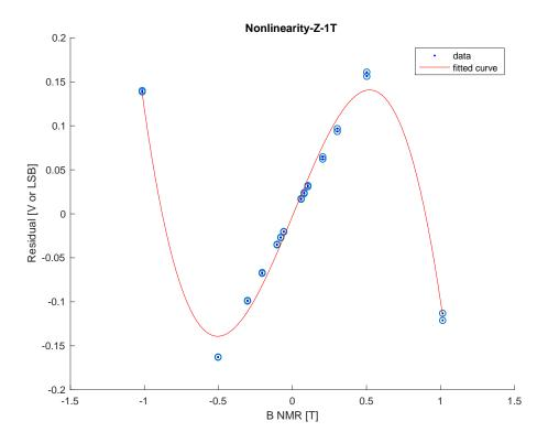
Figure 4. Typical nonlinearity plot, VCC = 3.3 V
