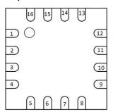
The functions of the pins differ according to the mode of operation, analog or digital – see Table 3 and Table 4. Unused pins can be left unconnected; the internal pull-down resistor is ~100 k $\Omega$ .
