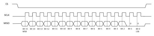
Figure 17. Timing of the data out when the resolution set to 14 bits.
