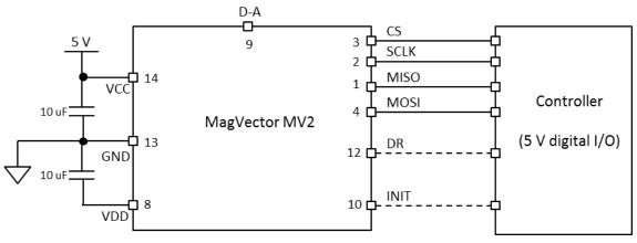
Figure 9. Circuit for sensor control and reading – digital mode
