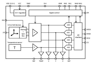
Figure 1. Block diagram
