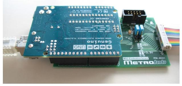
Figure 20. Arduino/Genuino UNO connected to MagVector MV2 test board.
