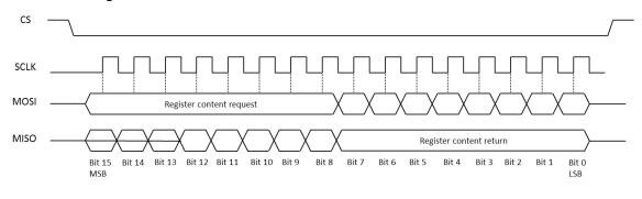
Figure 13. Timing diagram of the register read back
