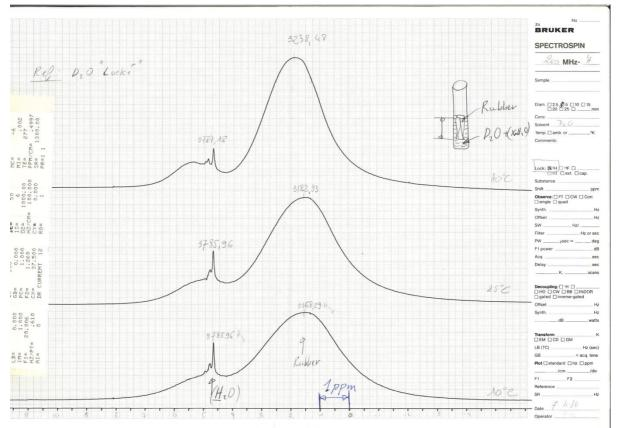
The hand-drawn sketch explains what was in the spectrometer's sample tube: a piece of isoprene rubber ( $CH_2=C(CH_3)-CH=CH_2$ ), bathed in heavy water ( $D_2O$ ) and a trace of regular water ( $H_2O$ ). The NMR resonance of the deuterium (D) nuclei serves as a reference, to lock the NMR spectrometer's RF generator. The spectrometer then accurately measures the NMR resonance spectrum of the Hydrogen (H) nuclei in both rubber and water.
