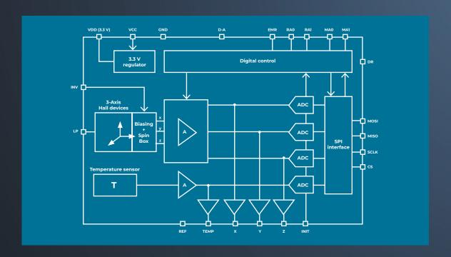
The MagVector™ MV2 allows you to integrate a sophisticated magnetometer into your electronic system. A typical application is a sensor array for magnetic filed monitoring. The MV2 was developped by MPS Tech Switzerland Sàrl, in cooperation with Metrolab. Metrolab uses the same sensor in several of its products, and is now making this technology available to electronic systems designers.
