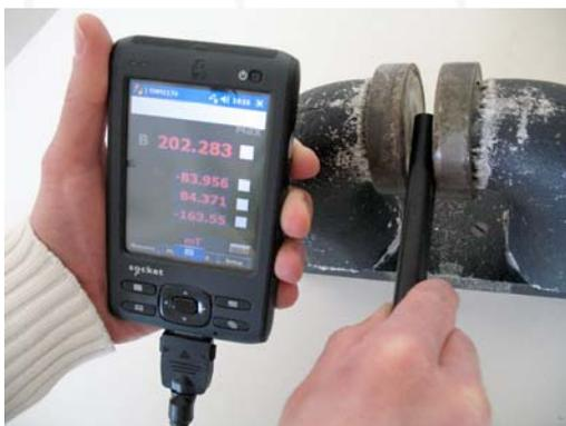
From the start, we conceived our new magnetometer as a portable instrument – this is why we wanted it to be so small and power-efficient. The user interface in this case would be provided by a commercially available handheld computer, or Personal Digital Assistant (PDA). PDAs provide a high-resolution color touch screen, powerful processor, local storage and high-density battery, all in a compact and attractive package and for a price that we could never match.
