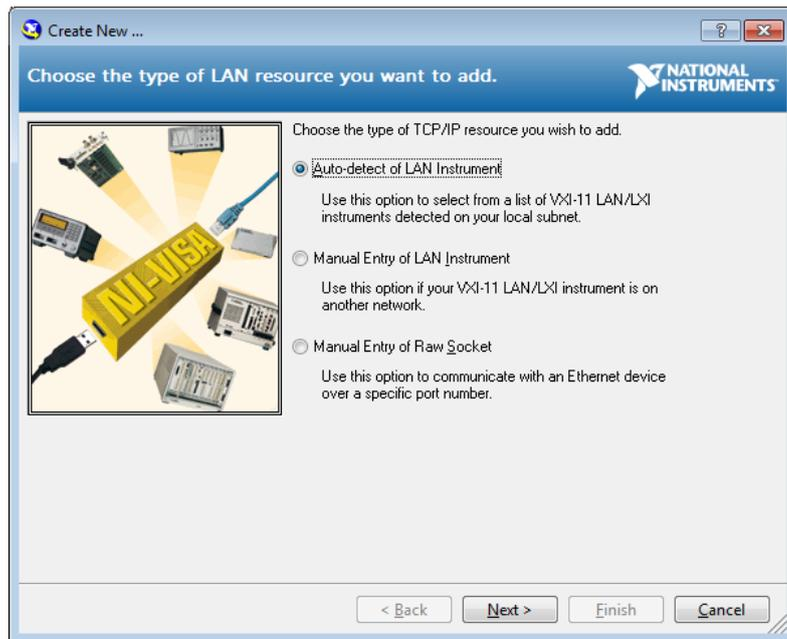
After having pressed the “Next” button, the system will search all VXI-11 compliant instruments over your sub-network. Once this operation is completed, a list of all instruments found on is displayed.
