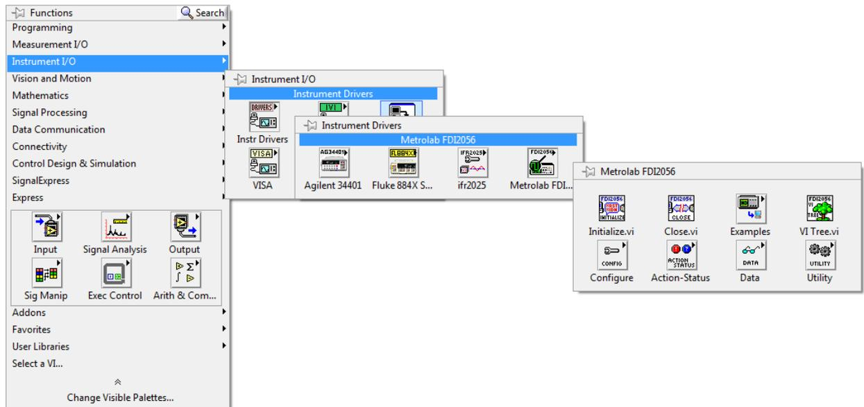
Choosing a VI from the “Example” sub menu is generally a good start. All examples are fully functional and configure some very basic and common measurements.
