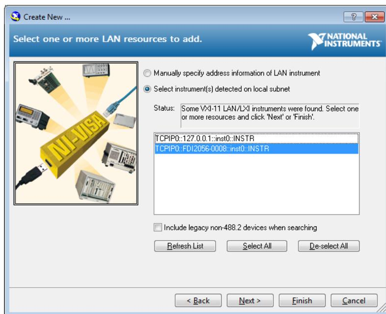
Select the FDI2056 by highlighting it on the list and then press the “Finish” button. You are now ready to communicate with the instrument.
