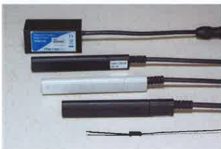
Figure 1 Family portrait of Metrolab's 3-axis magnetometers. The line encompasses probes for fields up to 14T or, using a Bartington Mag649, down to nano-teslas.
