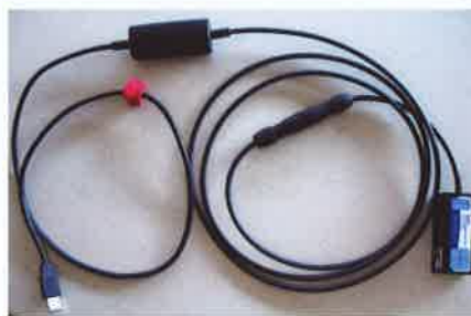
Figure 2 Metrolab's Three-axis Fluxgate Magnetometer, TFM1186. For simplicity, the differential receivers are on a second PCB, requiring a slightly larger housing than for the THM1176.
