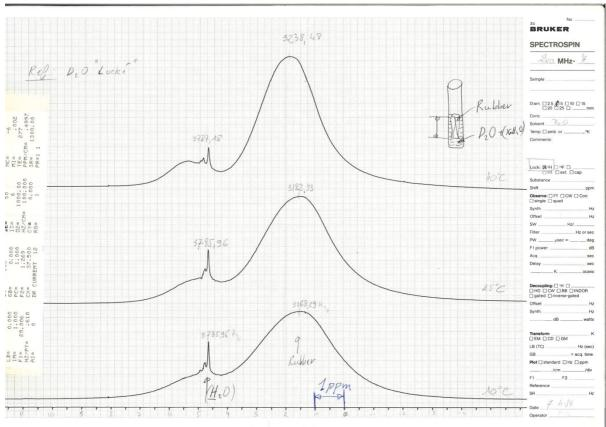
The hand-drawn sketch explains what was in the spectrometer's sample tube: a piece of isoprene rubber (CH<sub>2</sub>=C(CH<sub>3</sub>)-CH=CH<sub>2</sub>), bathed in heavy water (D<sub>2</sub>O) and a trace of regular water (H<sub>2</sub>O). The NMR resonance of the deuterium (D) nuclei serves as a reference, to lock the NMR spectrometer's RF generator. The spectrometer then accurately measures the NMR resonance spectrum of the Hydrogen (H) nuclei in both rubber and water.
