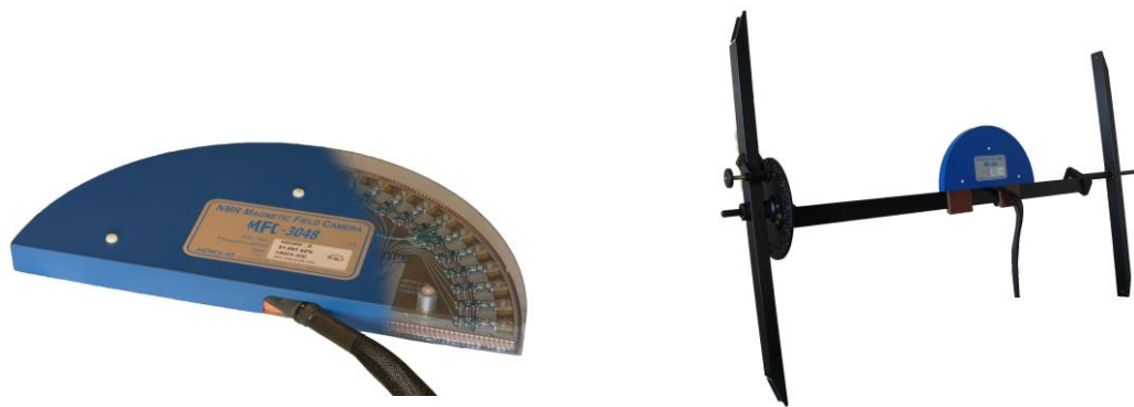
Figure 8. The Magnetic Field Camera probe array: (a) cut-away showing the probe positions; (b) as installed in a horizontal MRI magnet.
