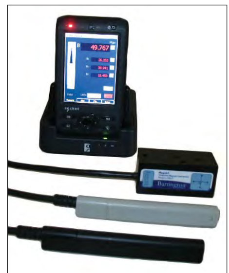
Figure 3. Family portrait: THM1176-HF (mT to 14 T), THM1176-LF ( \mu\text{T} to 8 mT) and TFM1186 (nT to 100 \mu\text{T} ).
