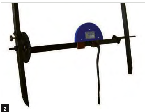
Figure 2: The magnetic field camera consists of an array of NMR probes (blue) mounted on a rotating jig. The jig's vertical supports are bolted to the magnet's cryostat, and the rotation is performed manually using a disk
