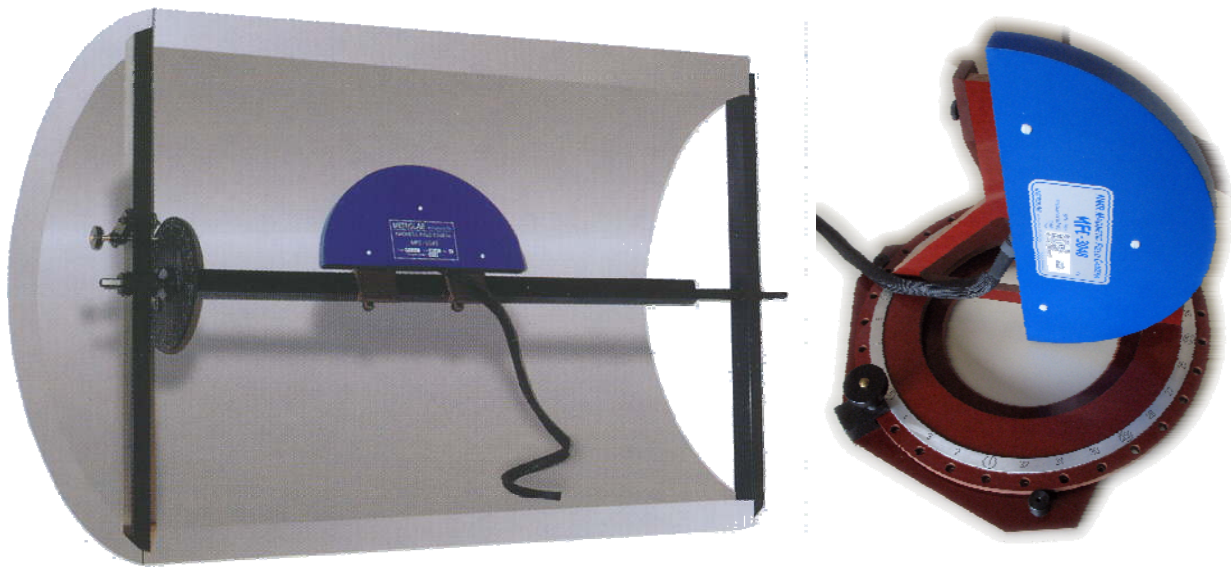
Figure 13. NMR mapping jigs for torroid- and C-shaped MRI magnets, respectively.
