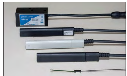
Figure 2. Three-axis magnetometer family portrait (top to bottom): Fluxgate probe for earth-field perturbations; High-Field probe for very strong fields; Low-Field probe for fringe fields; Medium-Field probe for general-purpose measurements; and High-Field Compact probe for narrow gaps.
