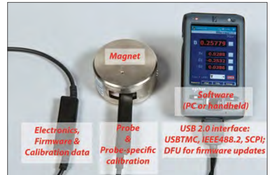
Figure 1. System Anatomy: the sensor, electronics and USB connector are little more than a cable with a few fat spots. The complexity resides in the firmware (embedded software) and host software. A calibration procedure unique to each sensor generates standardized calibration tables, written into flash memory in the electronics unit.
